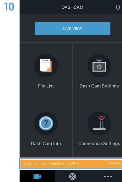
Return to the **THINKWARE CLOUD** app and check that "**Dash cam is connected via Wi-Fi**" is displayed at the bottom of the screen. The product is now connected to your Android device via Wi-Fi.
