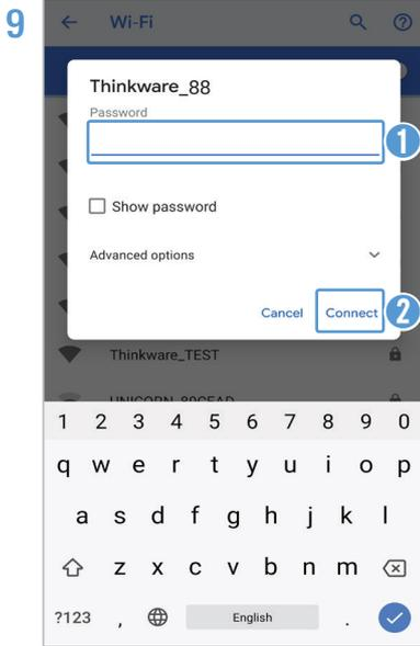
Enter "123456789" in the password field and tap **Connect**. The product is now connected to your Android device via Wi-Fi.
