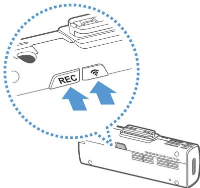
Press and hold the **REC** and Wi-Fi (📶) buttons simultaneously until you hear beeps.
