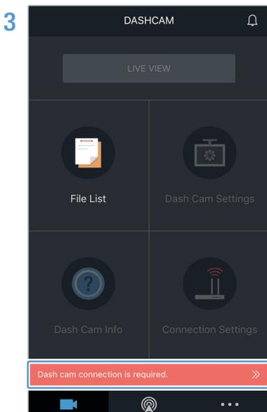
Tap **Dash cam connection is required** at the bottom of the screen.
